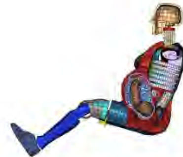
"Linda" by Volvo, a virtual pregnant crash-test dummy designed in 2002 by engineer Laura Thackray. "Linda" models the effects of high-speed impact on the womb, placenta, and fetus.
